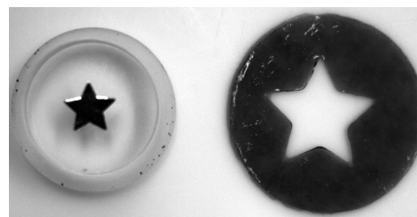
Figure 10. Photopatterned ePB 19.6 –PEO–11.5–0.5 hydrogel. The original mask on the quartz curing attachment (left) has been transferred to the hydrogel after UV curing. Swelling in water dissolved the uncured, masked region, resulting in excellent translation of the star pattern. Notably, the size of the star increases with swelling. The hydrogel was dyed for photographic clarity.
